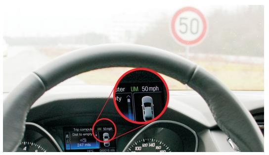
Speed Limiting Device in a vehicle
