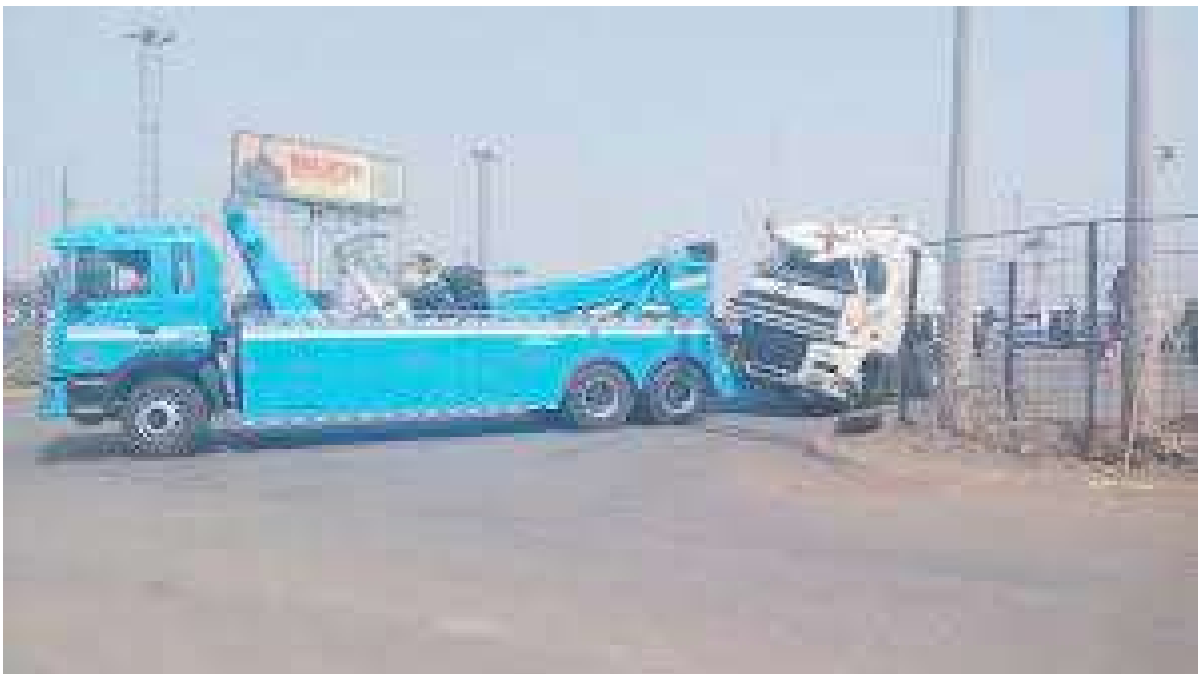
FRSC 70 tonnes recovery vehicle towing an accidental vehicle
